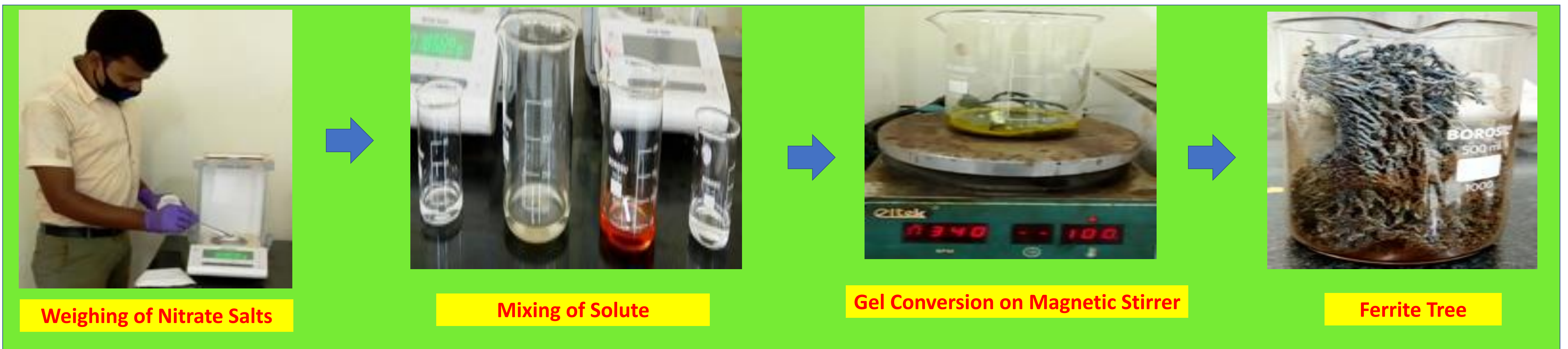
Flowchart of Preparation of Ferrite Magnetic Materials Tree in the Lab
